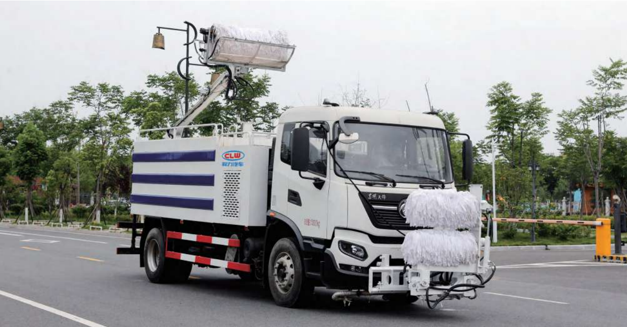
Dongfeng KR Tunnel Guardrail Cleaning Truck
