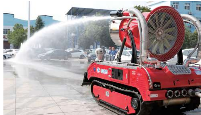
Smoke Extinguishing Vehicle
